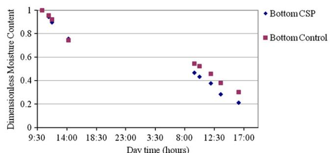
Fig. 15. Dimensionless moisture content during a simulated trial using the sun screen fabric for a two day period.
