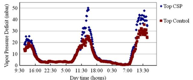
Fig. 10. Vapor pressure deficit for a three day period in each dryer using the burlap for simulated cloudy conditions.
